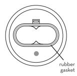
There is a rubber gasket under the battery door that may come out when replacing the batteries. This can easily be put back in the channel around the perimeter of the battery compartment before the battery door is closed back down.
